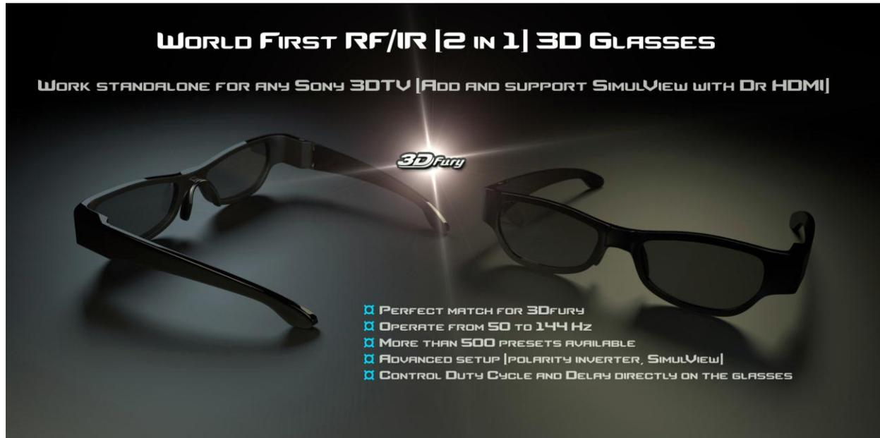
The 3Dfury glasses are very easy to operate there are 2 modes RF (Default) and IR. The glasses have 2 buttons: the mode key (Bottom Button) and the power key (Top Button). It also has a micro USB slot for charging the internal battery.
